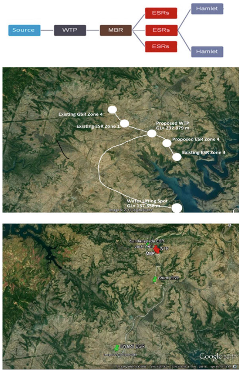
Fig. 3 Redesign of Khardi multivillage water supply scheme. a Schematic display of a water supply network components according to the planning protocol. b Replacement network and c alternate solution using Kundan dam as the source
